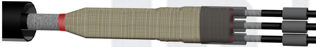
SLIDE THREE FINGERED GLOVE INTO POSITION
