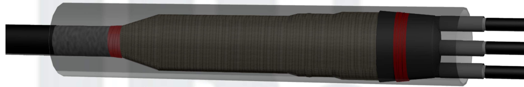
SLIDE OUTER RESIN TUBE INTO POSITION
