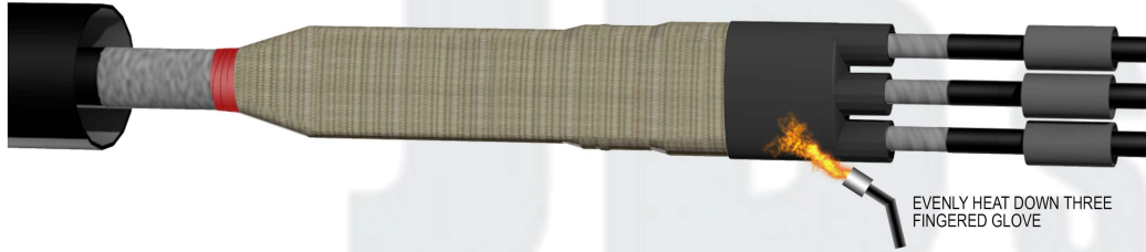
SLIDE THREE FINGERED GLOVE INTO POSITION
